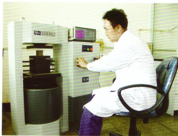
常温耐压测试机 Cold Crushing Strength Test Machine
