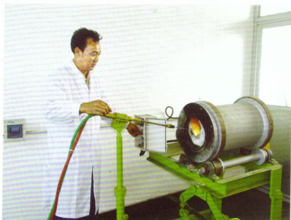
抗 渣 炉 Rotary corrosion Tester
